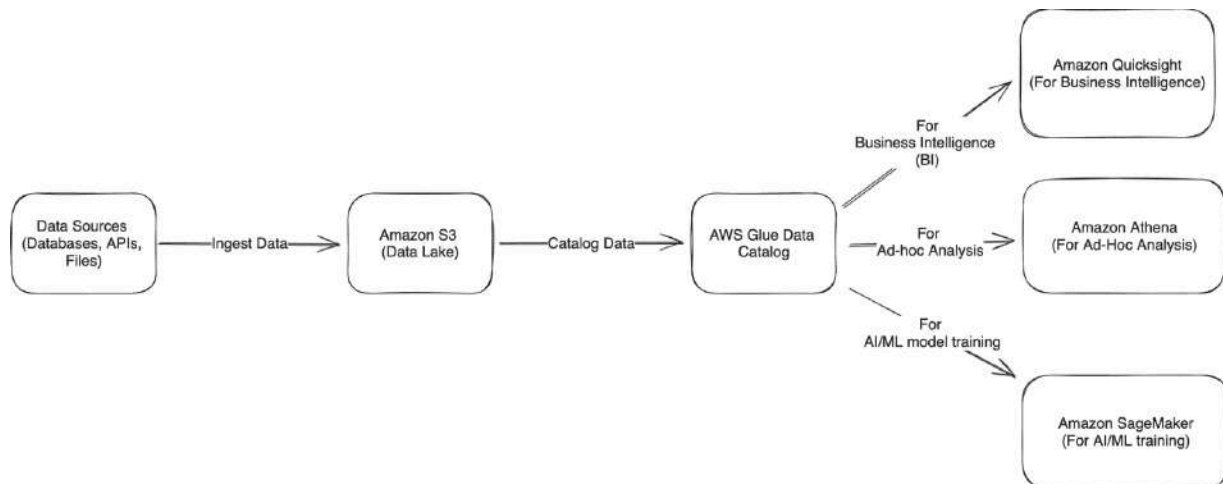
FIGURE 2.15 Data lake ingestion and processing pipeline
