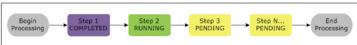
FIGURE 3.21 Step sequence execution and change of state
