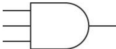
It's called a 3-input AND gate. The output is 1 only if all the inputs are 1. You can also create AND gates with many more inputs.
