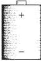
The voltage,  $E$ , is 1.5. That's a potential for doing work. But because the positive and negative terminals are connected solely by air, the resistance (the symbol  $R$ ) is very, very, very high, which means the current ( $I$ ) equals 1.5 volts divided by a large number. This means that the current is just about zero.
