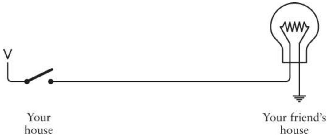
The V stands for *voltage*, but in a sense, it could also stand for *vacuum*. You can think of the V as an electron vacuum cleaner and think of the ground as an ocean of electrons. The electron vacuum pulls the electrons from the earth through the circuit, doing work along the way (such as lighting a lightbulb).
