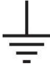
Electricians use this symbol because they don't like to take the time to draw an 8-foot copper pole buried in the ground. A circuit connected to this is said to be "connected to ground" or "grounded" rather than the more verbose "connected to *the* ground."
