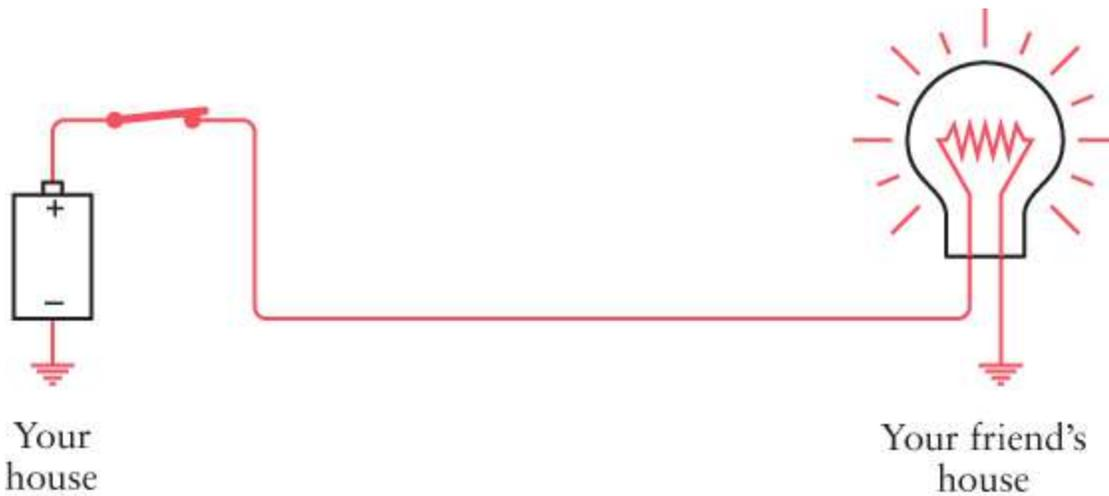
The electrons come out of the earth at your friend's house, go through the lightbulb and wire, pass through the switch at your house, and then go into the positive terminal of the battery. Electrons from the negative terminal of the battery go into the earth.
