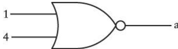
The output of this NOR gate is 1 except when the inputs are the 1 or 4 signals. For these two numbers, the top segment is *not* illuminated.
