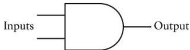
This is the first of six basic logic gates. The AND gate has two inputs and one output. You'll often see the AND gate drawn with the inputs at the left and the output at the right. That's because people who are accustomed to reading from left to right prefer reading electrical diagrams from left to
