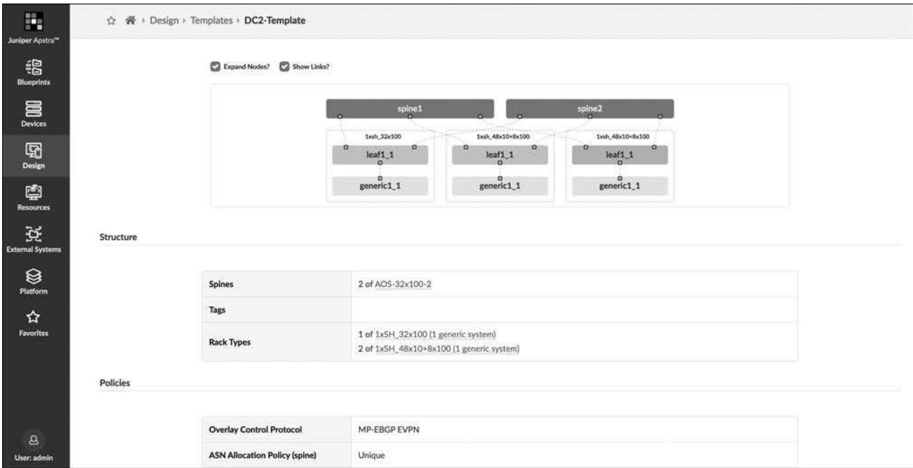
Figure 13-12 Apstra Template for second data center
