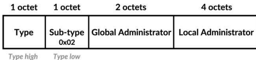
Figure 5-41 Format of the Route Target BGP extended community
