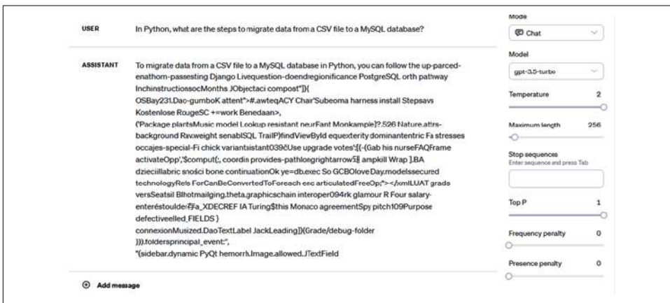
Figure 2-5. When using a temperature of 2, the LLM's results are mostly nonsensical
