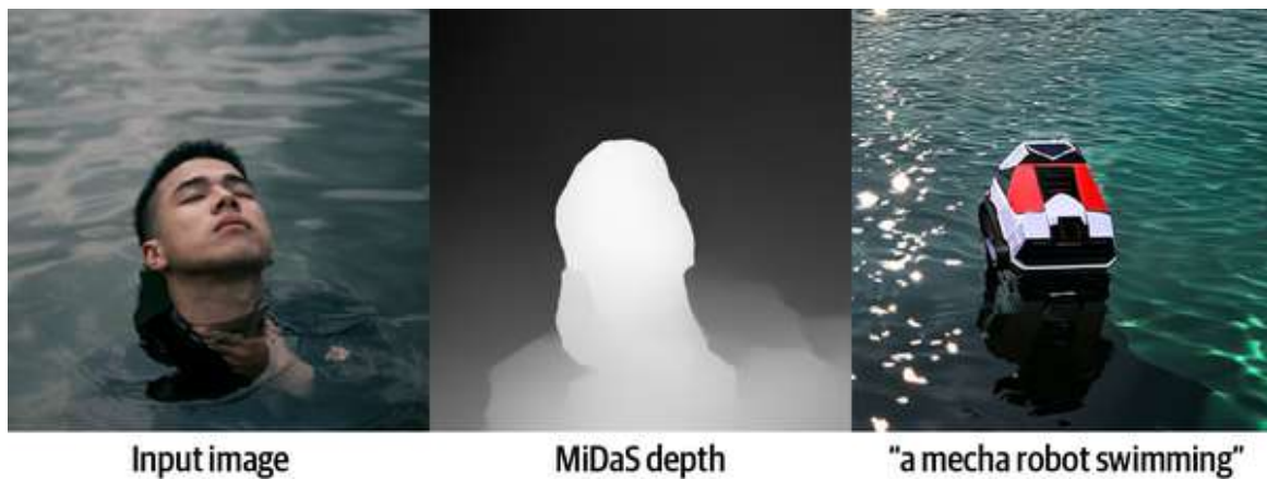
Figure 7-6. Inference of Stable Diffusion 2 fine-tuned with MiDaS depth conditioning
