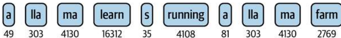
Figure 2-3. In this example of subword tokenization, llama is split into two tokens because it was likely not a common word in the data used to create the tokenizer
