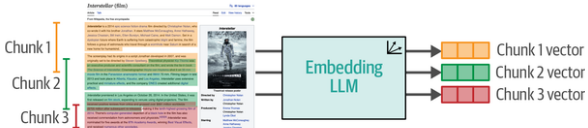
Figure 8-10. Chunking the text into overlapping segments is one strategy to retain more of the context around different segments.
