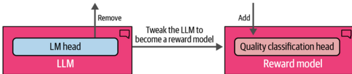
Figure 12-25. The LLM becomes a reward model by replacing its language modeling head with a quality classification head.
