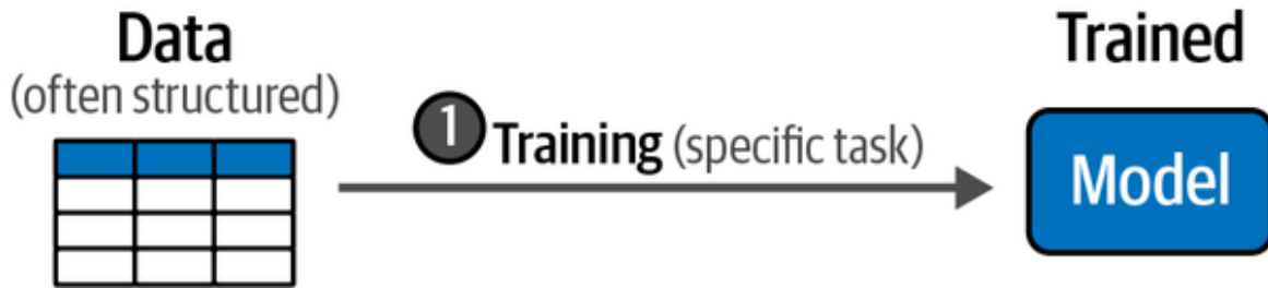
Figure 1-29. Traditional machine learning involves a single step: training a model for a specific target task, like classification or regression.
