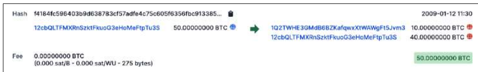
Figure 8-1. The first bitcoin transaction sent between two addresses, viewed in a public blockchain explorer
