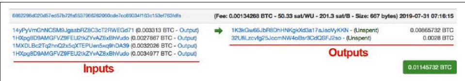
Figure 2-2. A sample transaction, and how it looks in a Bitcoin block explorer
