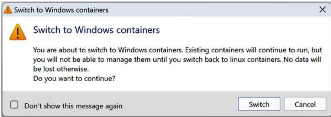
Figure 5-2. Switch to Windows containers confirmation
