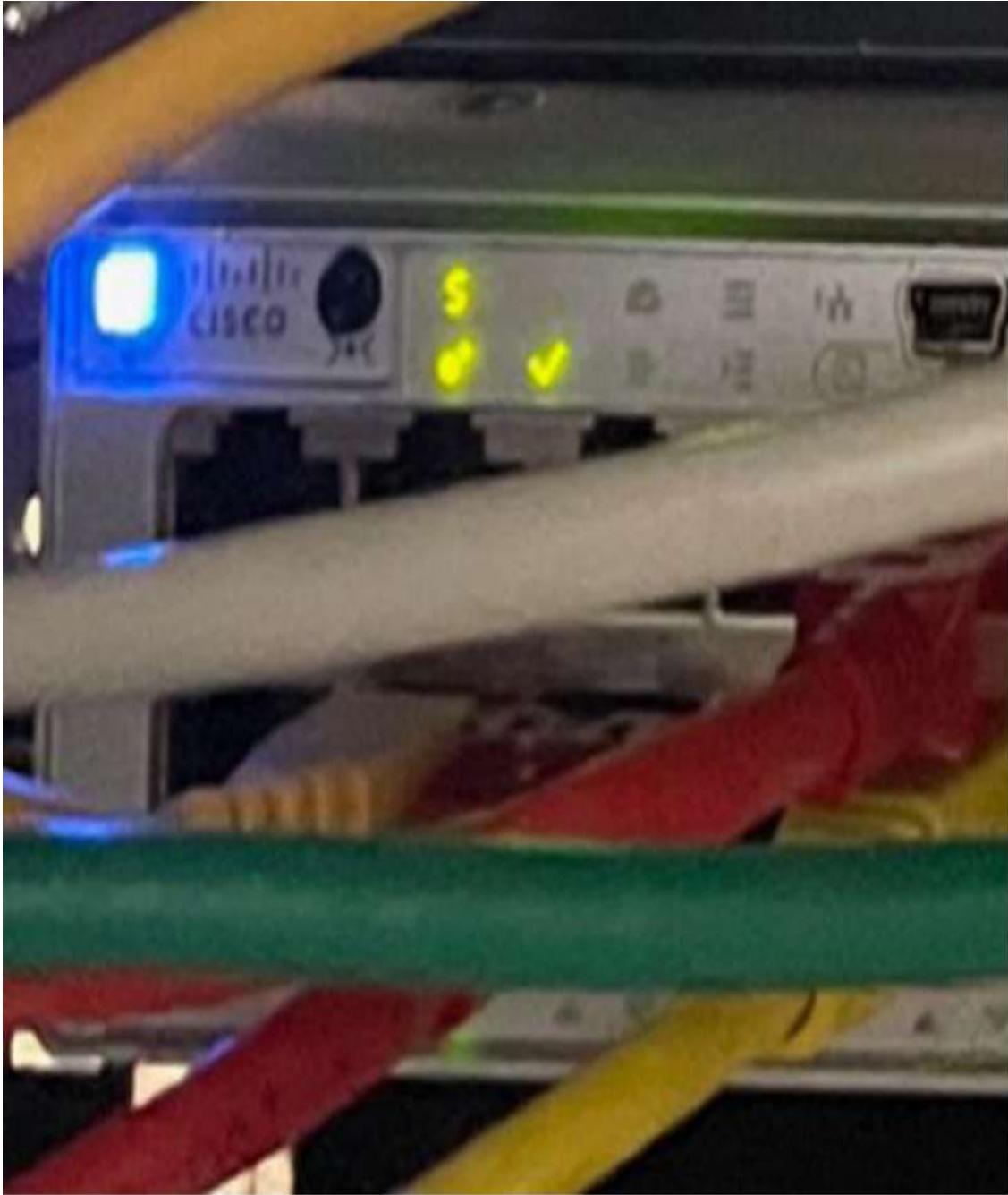
Figure 7-29 Blue Configurable Beacon on a Catalyst 9300 Series Switch
