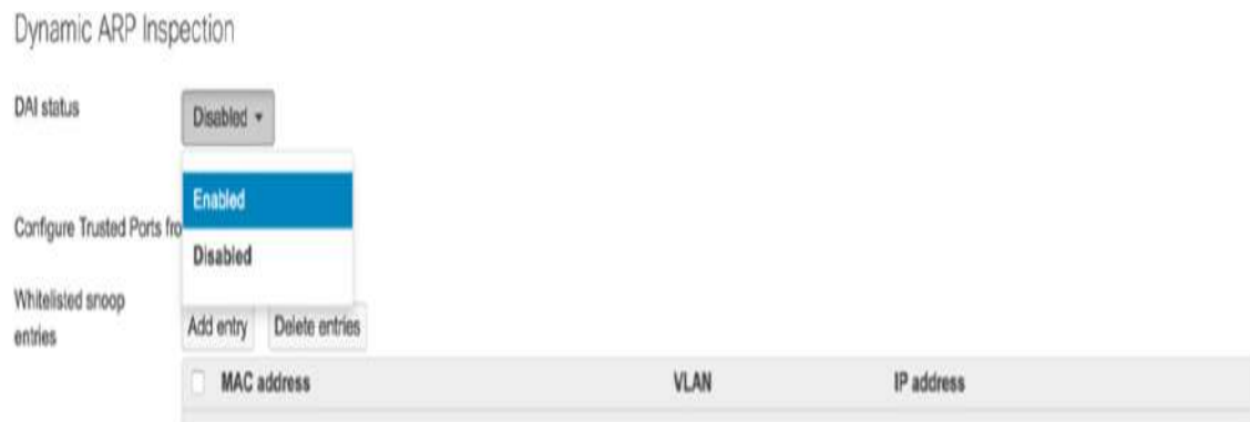
Figure 9-14 Dynamic ARP Inspection (Meraki)
