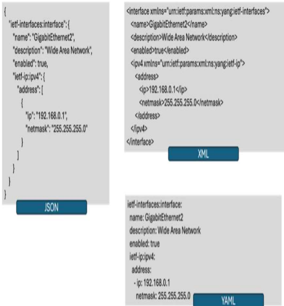
Figure 2-6 IPv4 Interface Definition in JSON, XML, and YAML
