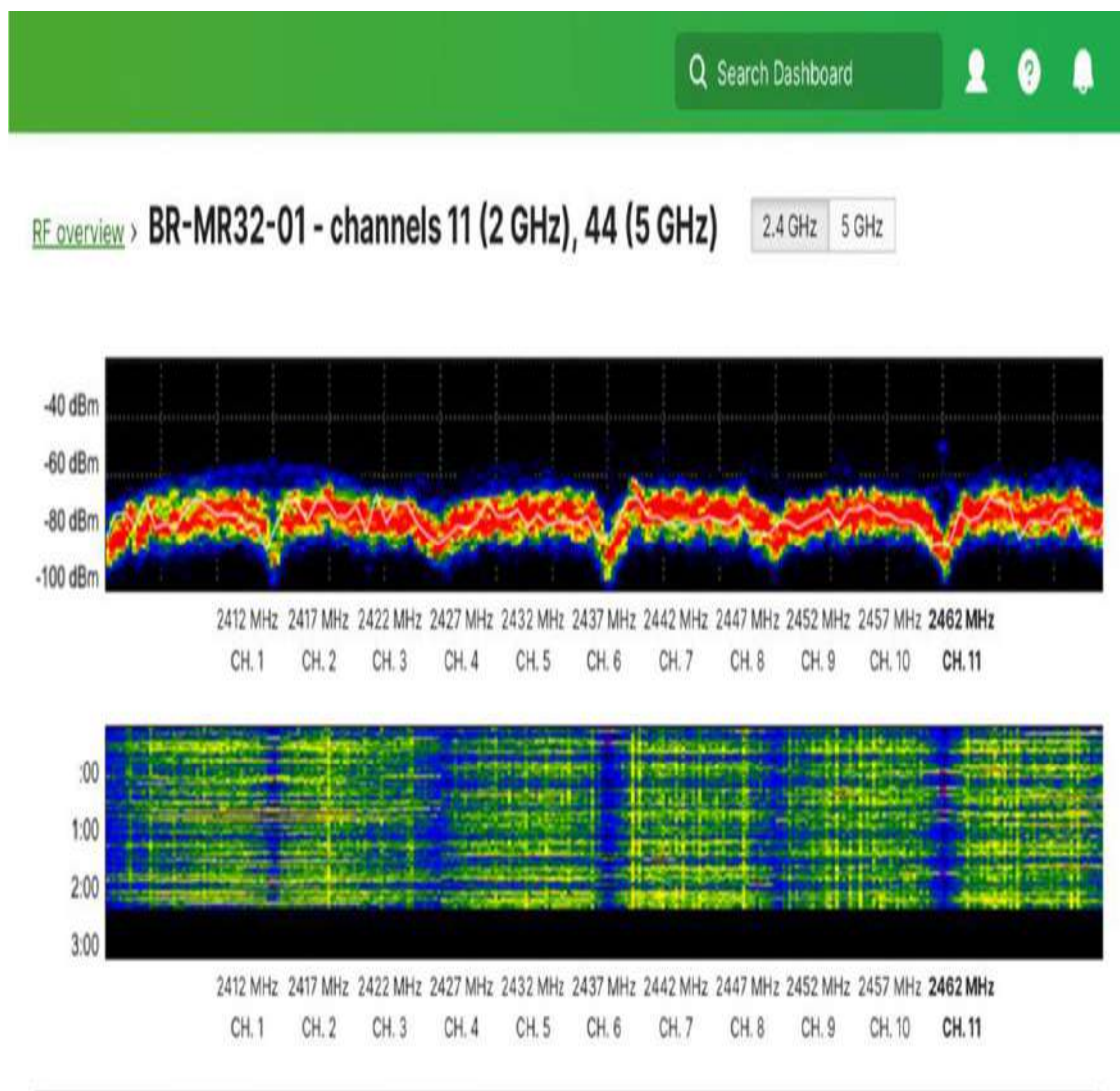
Figure 13-12 Meraki Dashboard Spread Spectrogram
