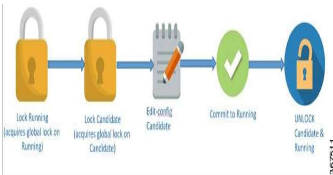
Figure 23-1 Locking and Unlocking Candidate and Running Configurations During Provisioning
