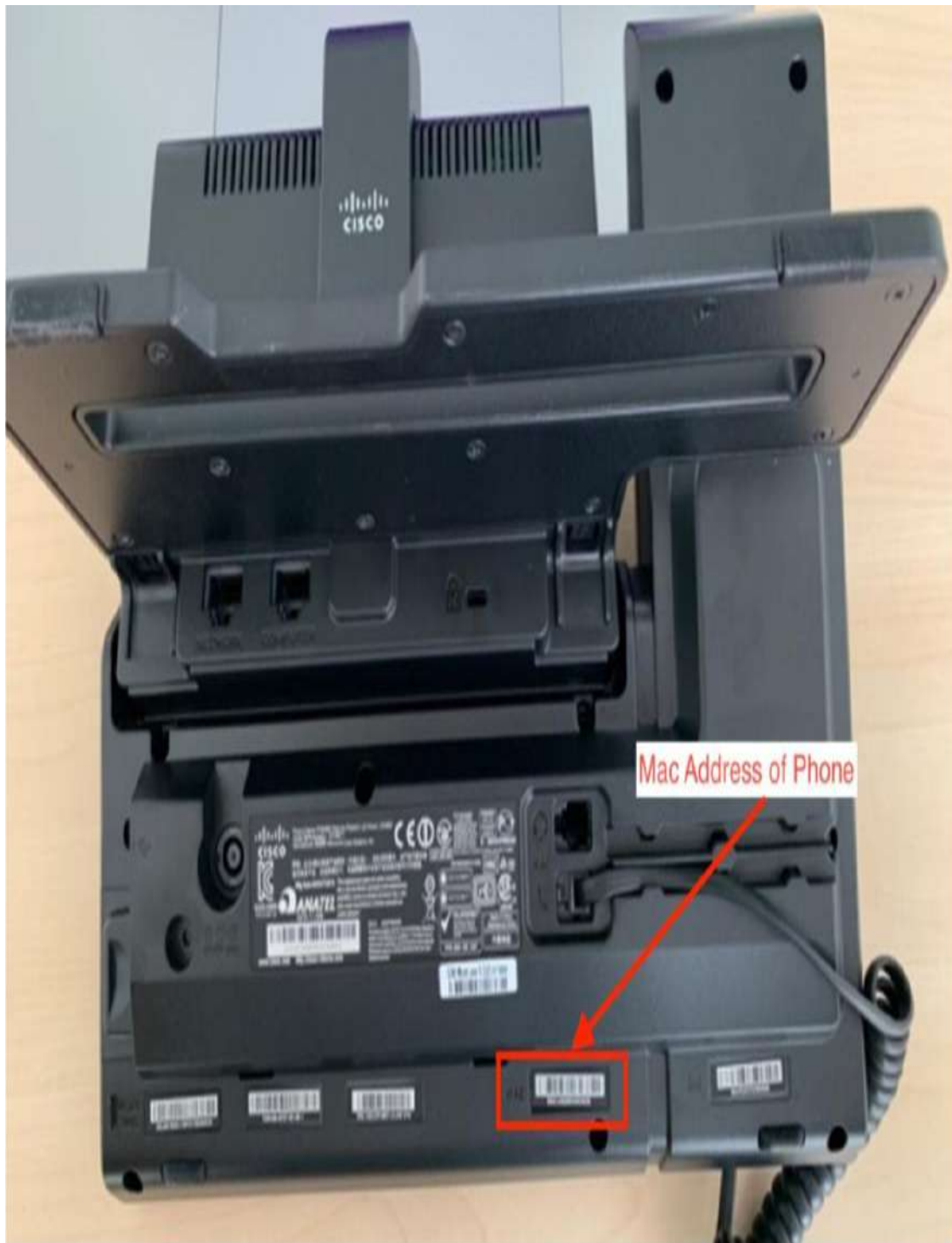
Figure 9-12 Visible MAC Address on Rear of IP Phone
