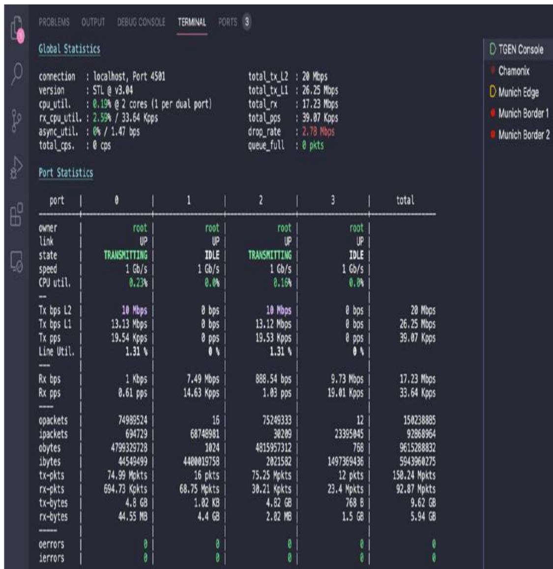
Figure 11-23 Packet Drops Observed in TRENDS
