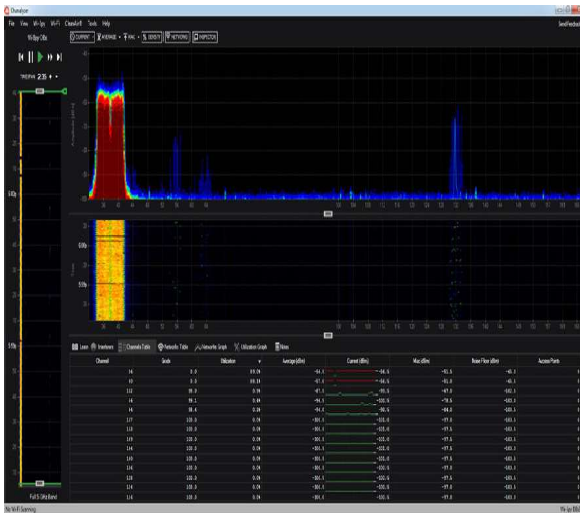
Figure 13-13 Jammed RF Channel
