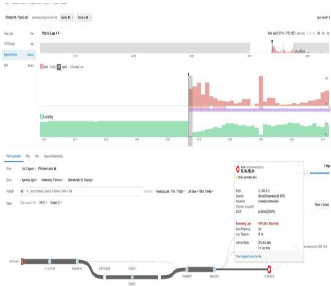
Figure 11-7 ThousandEyes Dashboard: Showcasing Network Loss Toward a Remote Service
