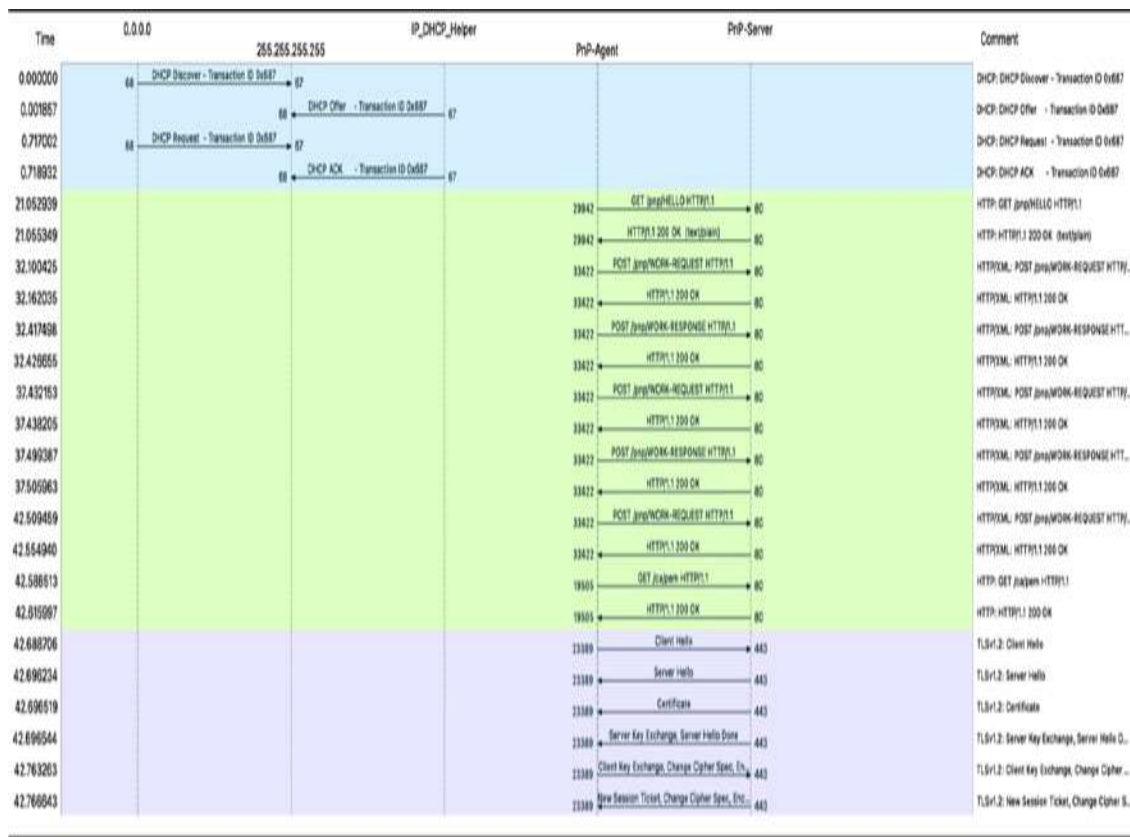
Figure 7-2 Wireshark PnP Flow Graph
