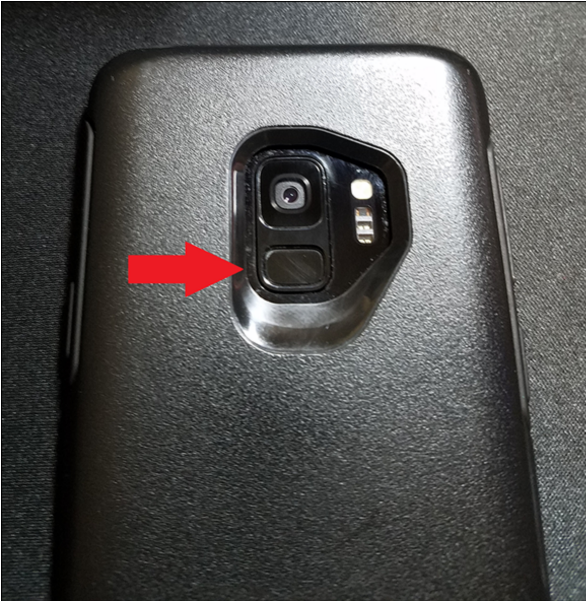
FIGURE 8-3: A phone fingerprint sensor on a Samsung Galaxy S9 in an Otterbox case. Some phones have the reader on the front, whereas others, like the S9, have it on the back.
