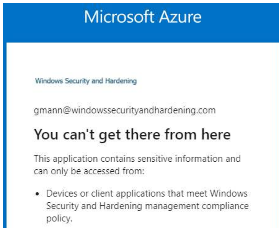
Figure 8.26 – Access blocked to the Azure portal
