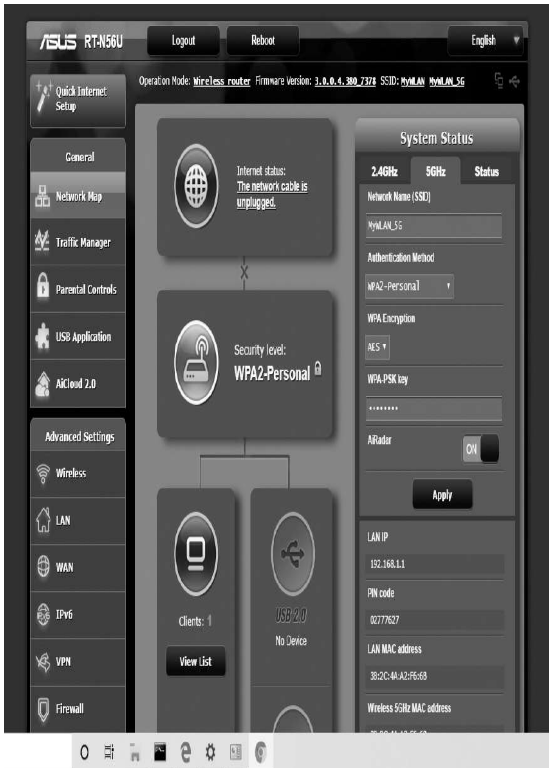
FIGURE 5-9 The initial configuration screen on an ASUS wireless router. Courtesy of Asus.
