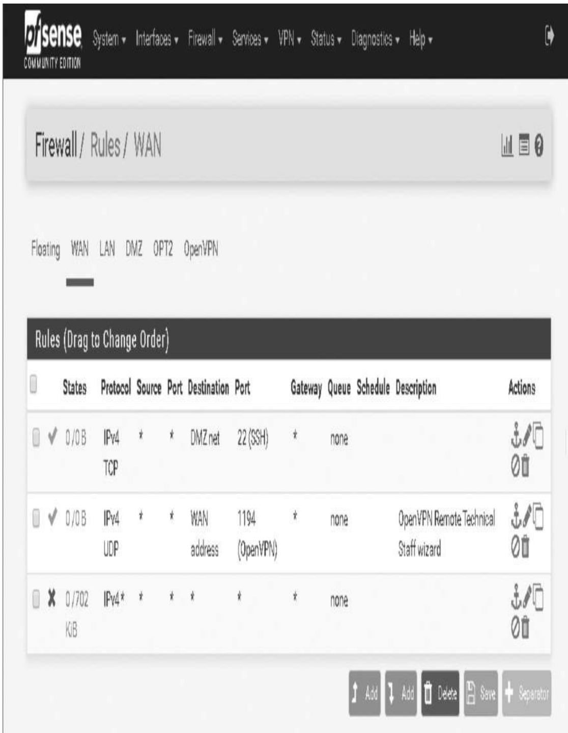
FIGURE 8-1 pfSense’s default rule configuration interface, showing a default deny as the last rule. © pfSense
