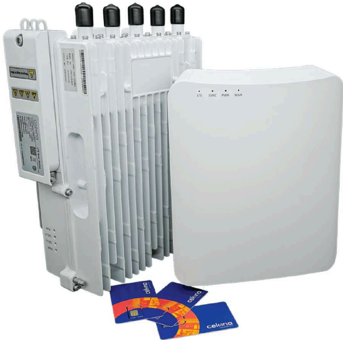
Figure 8.16: Cellular nodes (or cellular APs) look and operate very much like Wi-Fi APs. Pictured here are two models from Celona, one outdoor and one indoor, along with SIM cards.
