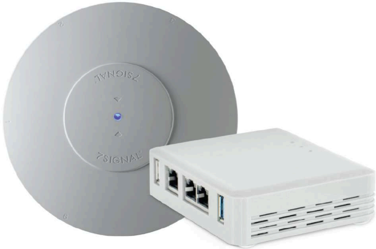
Figure 7.21: Vendor 7Signal offers an app-based agent and hardware sensors including a permanent fixture model that looks like a small AP and a more portable device.
