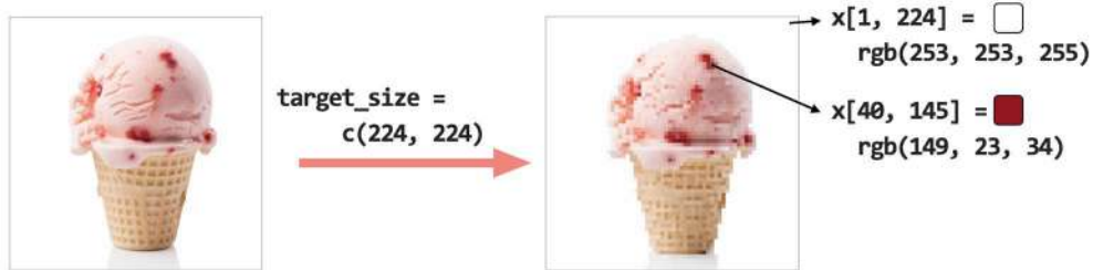
Figure 15.4: The picture of ice cream has been reduced from a matrix of 1,000x1,000 pixels to 224x224; each pixel in the image has three color channels
