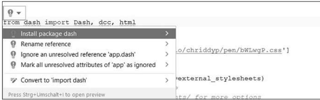
Figure 2-7: Installing Dash through PyCharm
