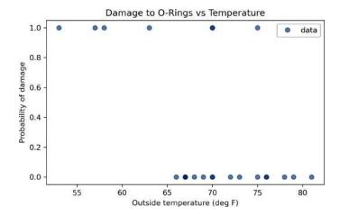
When the outside temperature was below 65 degrees F, there was always damage to the O-rings. When the temperature was above 65 degrees F, there was usually no damage.
