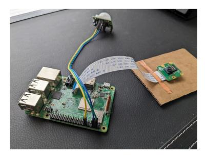
With the hardware fully assembled and the Pi powered up, it's time to write some Go code to detect motion whenever you wave your hand near the PIR.
