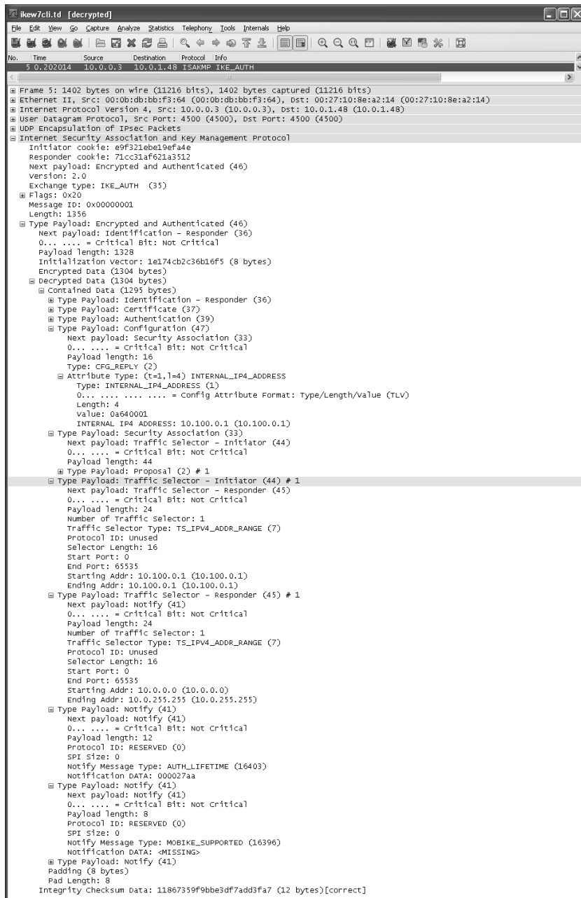
Figure 18-25 Completing the IKE_AUTH exchange, the responder produces an Encrypted/Authenticating data payload containing the following payloads: Identification responder (IDr), CERT, AUTH, CP(CFG_REPLY), SA, narrowed TSi and TSR, along with N(AUTH_LIFETIME), N(MOBIKE_SUPPORTED), and N(NO_ADDITIONAL_ADDRESSES). The first CHILD_SA can now commence.
