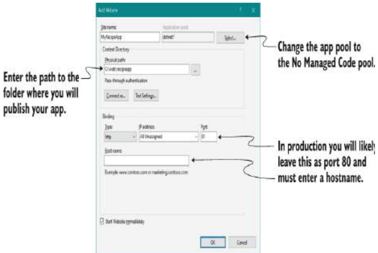
Figure 27.6 Adding a new website to IIS for your app. Be sure to change the Application Pool to the No Managed Code pool created in the previous step. You also provide a name, the path
