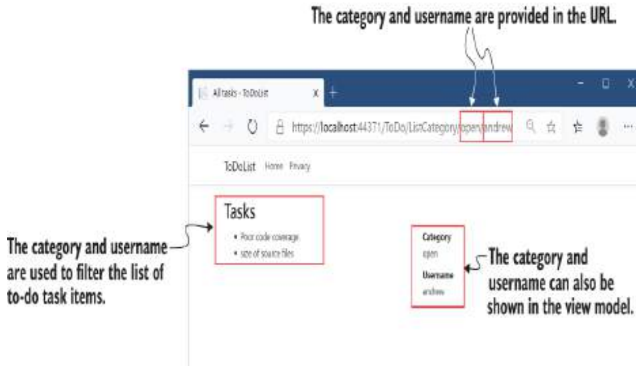
Figure 16.1 A basic to-do list application that displays to-do list items. A user can filter the list of items by changing the category and username parameters in the URL.
