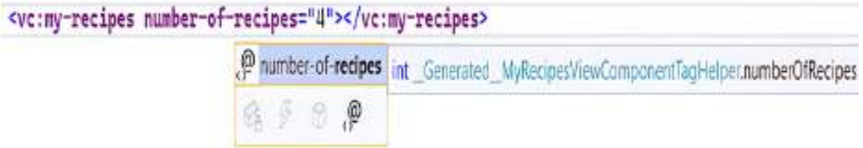
Figure 32.5 Visual Studio provides IntelliSense support for the method parameters of a view component's InvokeAsync method. The parameter name, in this case numberOfRecipes , is converted to kebab-case for use as an attribute in the Tag Helper.
