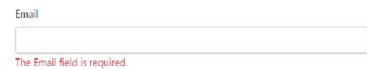
Figure 18.8 Validation messages can be shown in an associated <span> by using the Validation Message Tag Helper.
