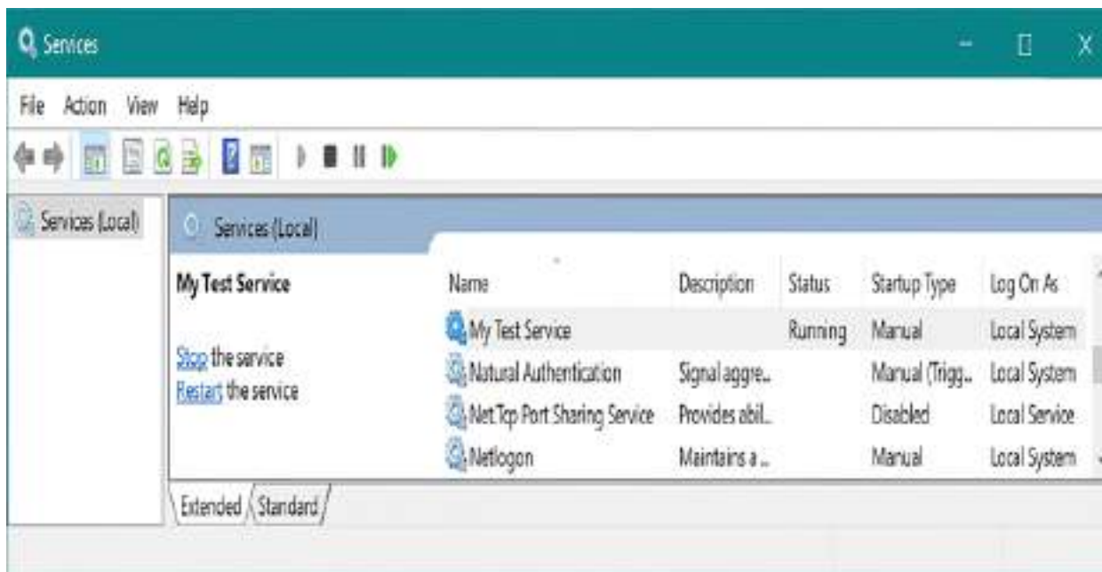
Figure 34.3 The Services control panel in Windows. After installing a worker service as a Windows Service using the sc utility, you can manage your worker service from here. This control panel allows you to control when the Windows Service starts and stops, the user account that the application runs under, and how to handle errors.
