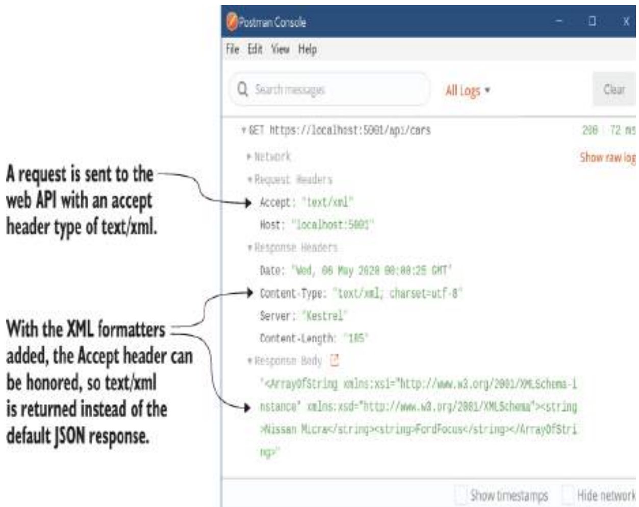
Figure 20.8 With the XML output formatters added, the Accept header's text/xml value is respected, and the response is serialized to XML.
