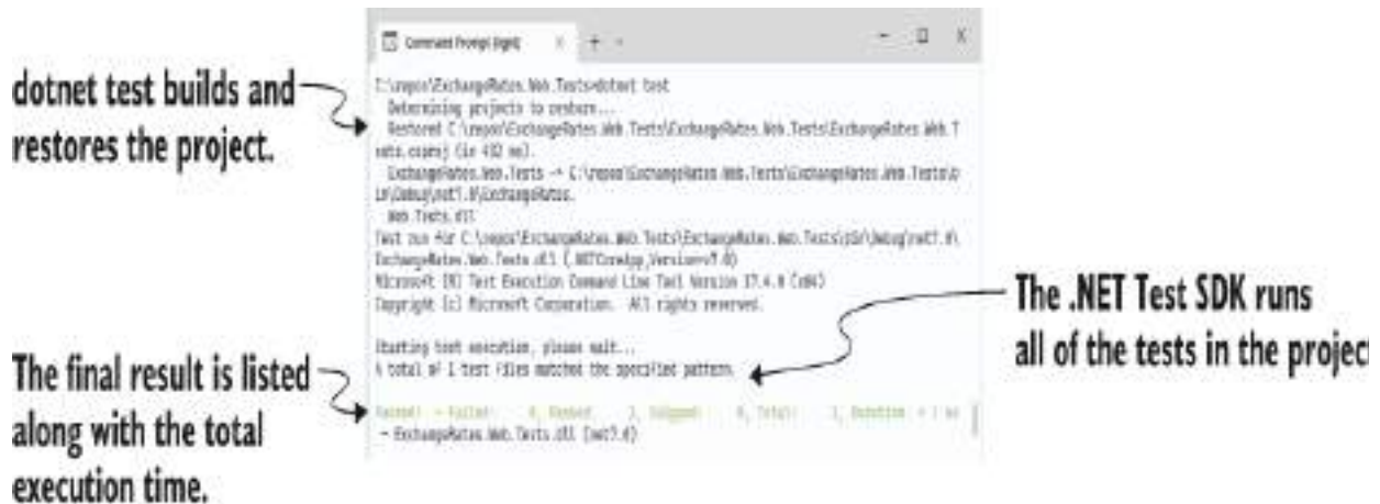
Figure 35.3 You can run tests from the command line using dotnet test . This restores and builds the test project before executing all the tests in the project.
