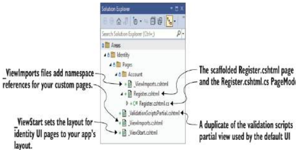
Figure 23.13 The scaffolder generates the Register.cshtml Razor Page, along with supporting files required to integrate with the remainder of the default Identity UI.
