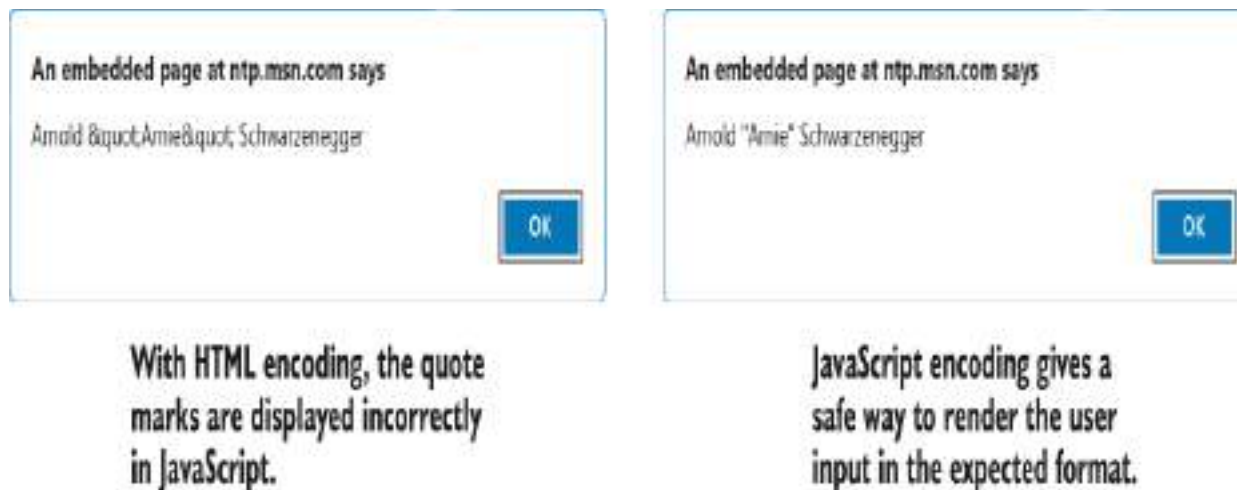
Figure 29.3 Comparison of alerts when using JavaScript encoding compared with HTML encoding
