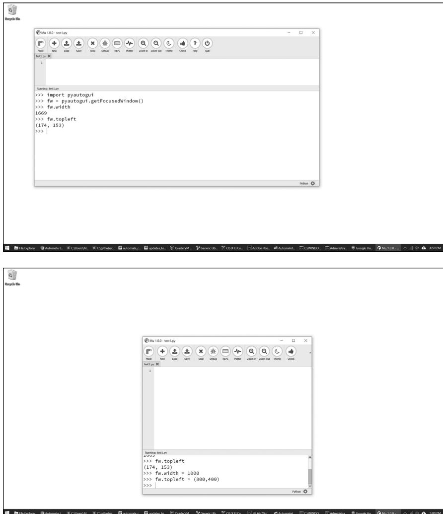
Figure 23-5: The Mu Editor window before (top) and after (bottom) using the Window object attributes to resize and move it
