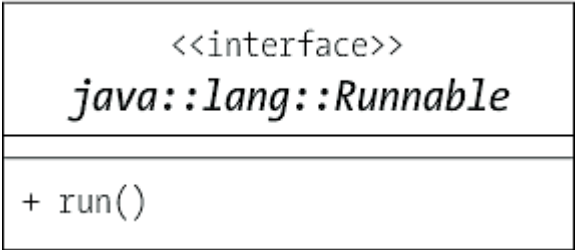
Figure 17.3 Unified Modeling Language (UML) Diagram of the Simple Runnable Interface
