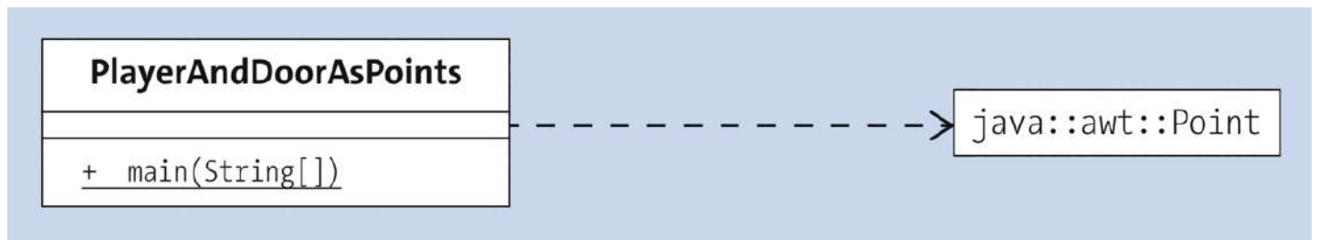
Figure 3.4 UML Diagram Showing the Dependency between a Class and java.awt.Point with a Dashed Line. Attributes and Operations of the Point Object Are Not Shown.
