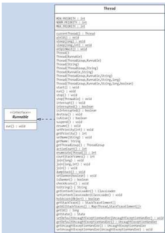
Figure 17.4 UML Diagram of the Thread Class Implementing Runnable
