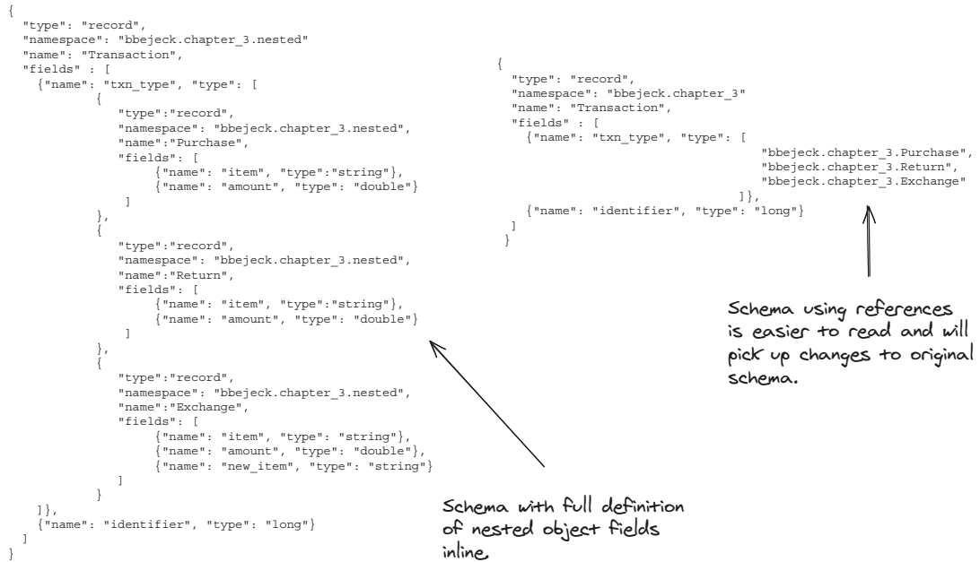
Figure C.1 Comparing a schema with nested records vs. using schema references
