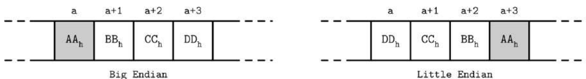
Figure 3-1. Big- and little-endian byte order. The most significant byte is shown in gray. Addresses, denoted by a , grow from left to right.
