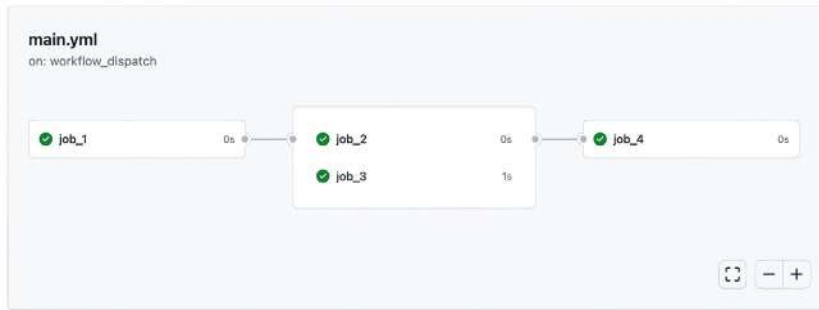
Figure 3.4 A visual representation of chained workflow jobs in GitHub
