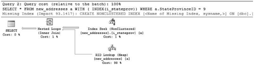
Figure 19-9 Graphical execution plan for the query in Example 19.13
