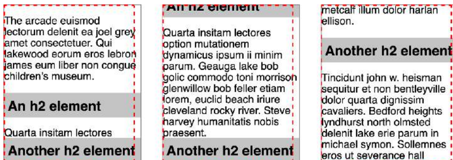
Figure 10-56. Sticking to the bottom of the sticky-positioning rectangle
