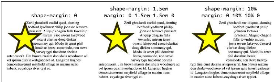
Figure 20-35. Making sure the shape margins don't get clipped
