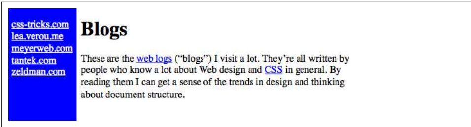
Figure 2-17. Using descendant selectors to apply different styles to the same type of element
