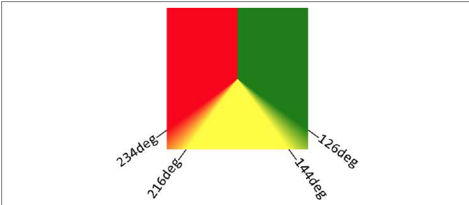
Figure 9-45. Conic gradients with solid-color wedges and smooth transitions
