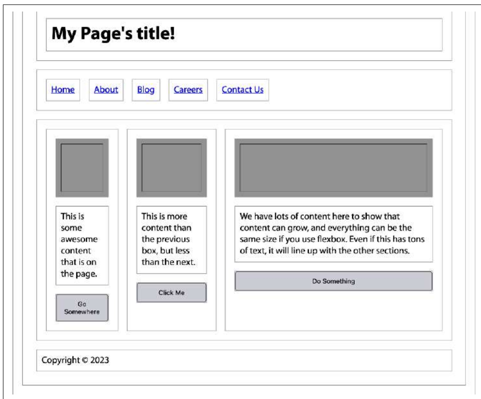
Figure 11-7. Home page layout using flex-direction: row and column ▶
