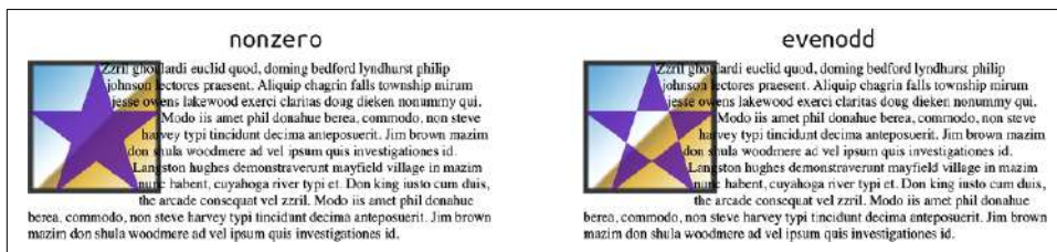
Figure 20-32. The two polygonal fills
