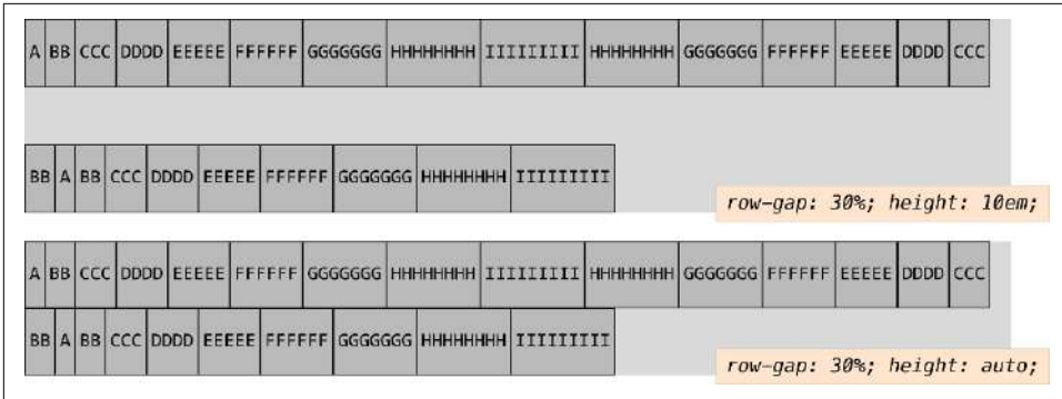
Figure 11-34. Percentage-based row gaps with and without explicit container heights
