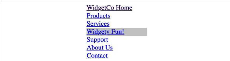
Figure 6-2. Changing the display role from inline to block
