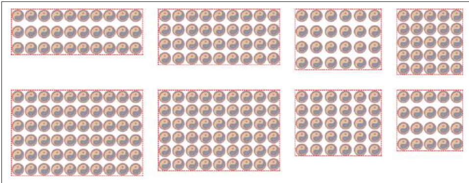
Figure 8-26. Tiling with different intervals showing background-repeat: space on elements of different sizes
