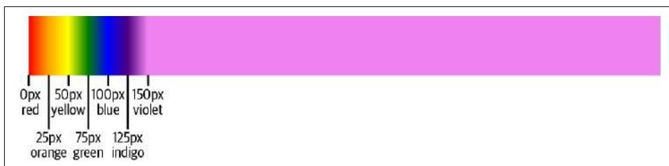
Figure 9-6. Placing color stops every 25 pixels
