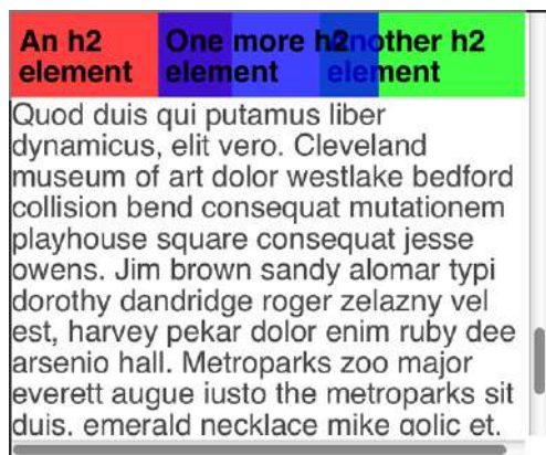
Figure 10-58. A sticky-header pileup
