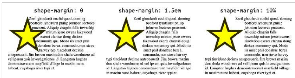
Figure 20-34. Adding margins to float shapes
