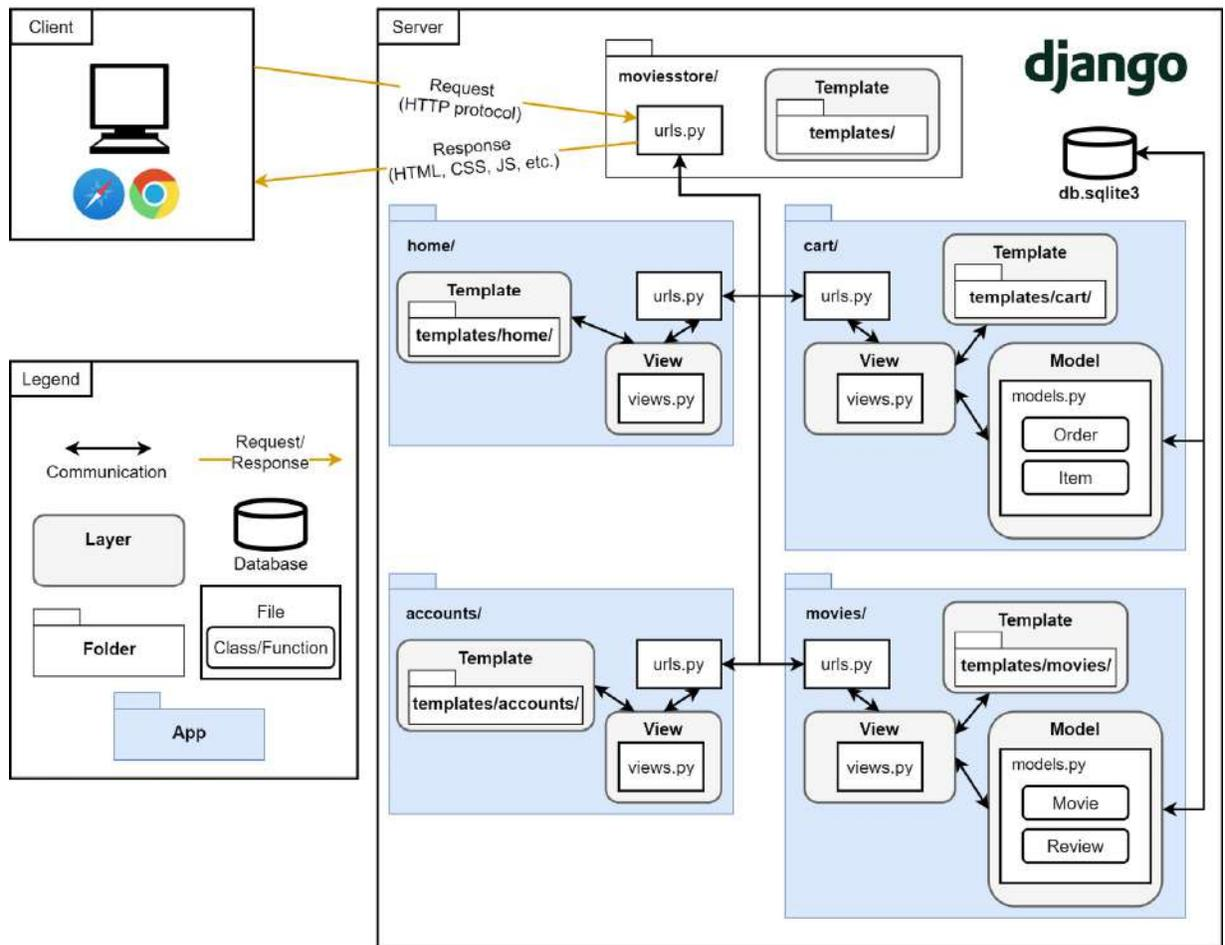
Figure 1.11 – The Movies Store software architecture diagram
