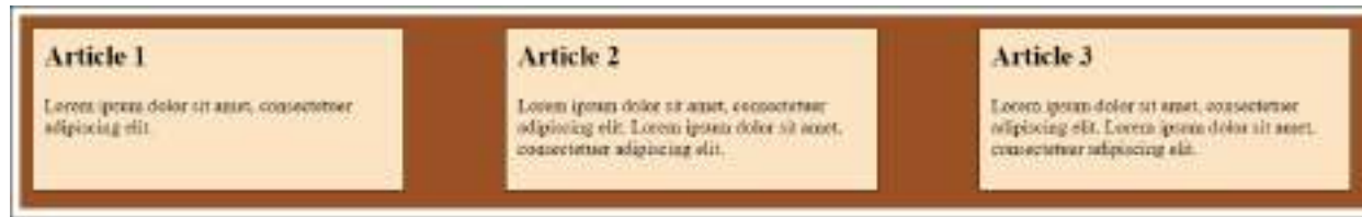
Figure 12.35 “justify-content: space-between;” Makes Sure That the Elements Are Arranged with Equal Spaces In Between: The First and Last Elements Are Located at the Beginning and End of the Line, Respectively
