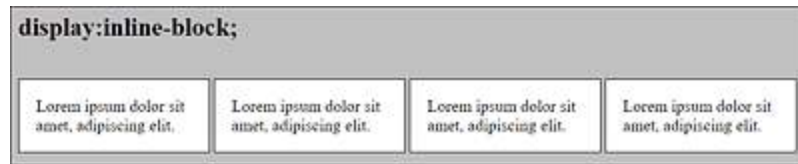
Figure 13.49 Here, I've Set the Behavior of the <p> Elements to “ display:inline-block; ”
