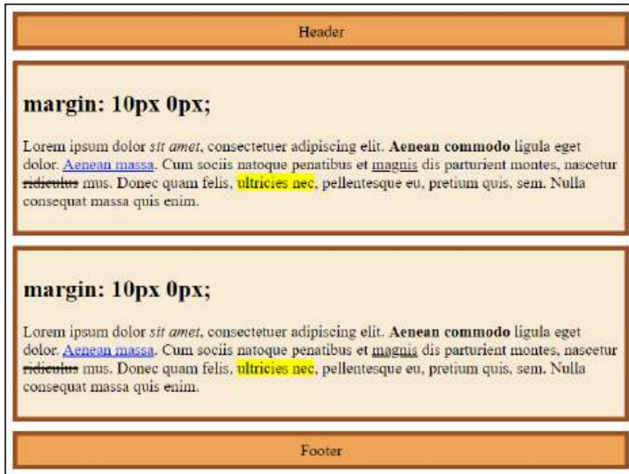
Figure 11.7 The <article> Element Has Been Set with an Outer Margin of 10 Pixels to the Top and Bottom (“margin: 10px 0px”)
