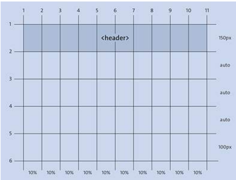
Figure 13.37 The <header> Element Was Added to the Grid Layout
