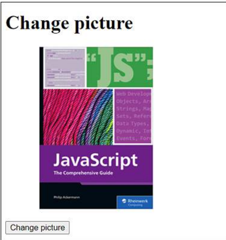
Figure 19.11 In This Example, the “src” and “old” Attributes of the <img> Element Are Changed So the Image Gets Replaced
