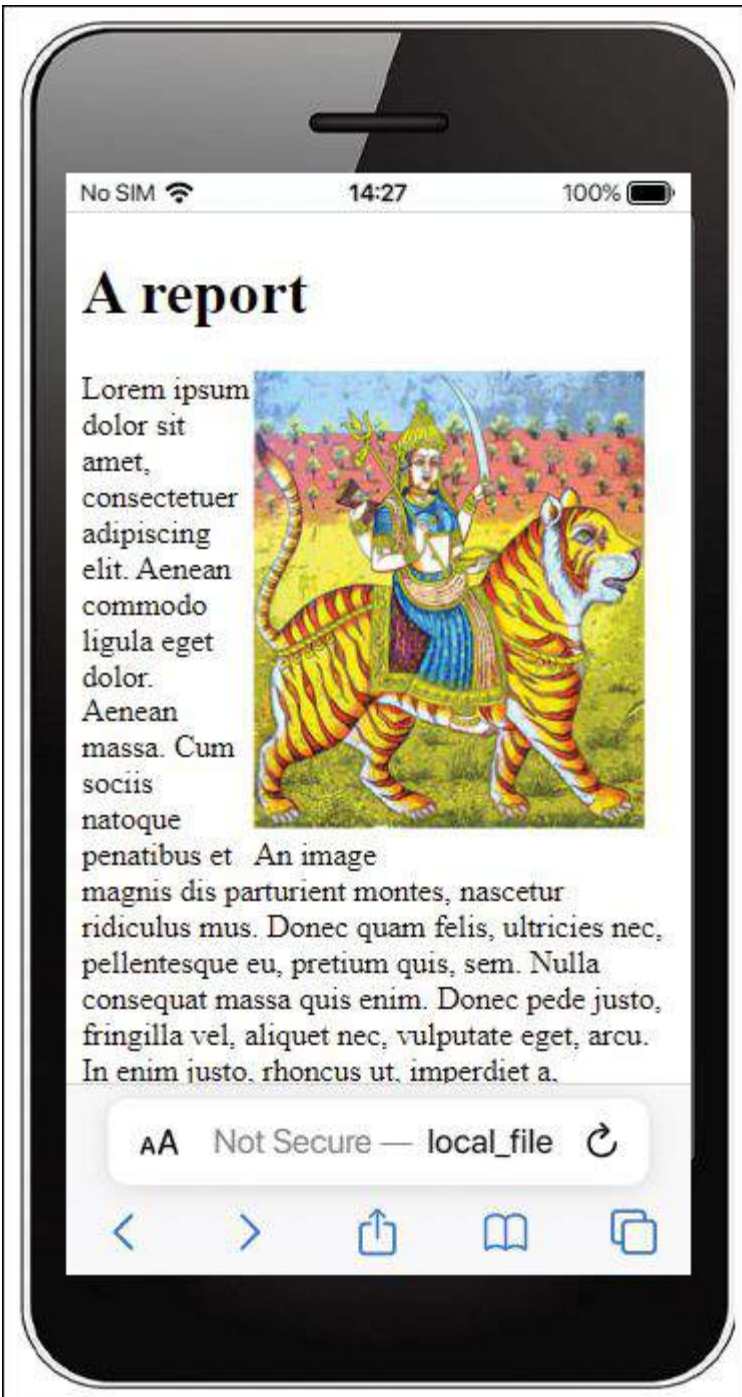
Figure 12.21 Layout No Longer Looks Nice on a 320-Pixel-Wide Smartphone: In Some Places, There's Only One
