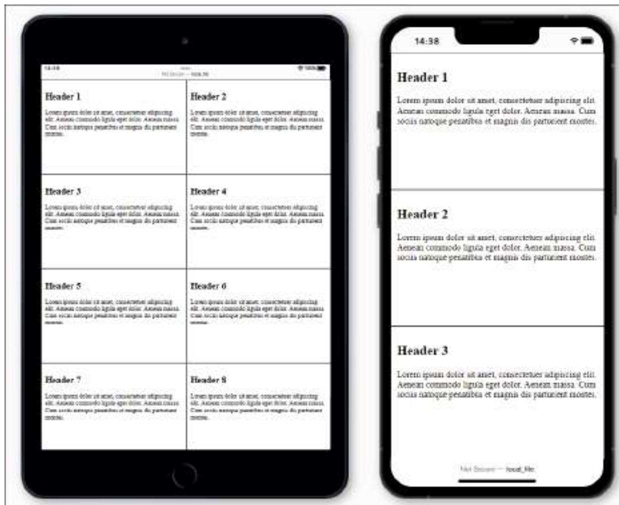
Figure 13.52 A Two-Column Layout with “width: calc(100% / 2);” for a Viewport of Less Than 640 Pixels (Left) and a Single-Column Layout with “width: 100%;” for the Viewport of Less Than 480 Pixels (Right)
