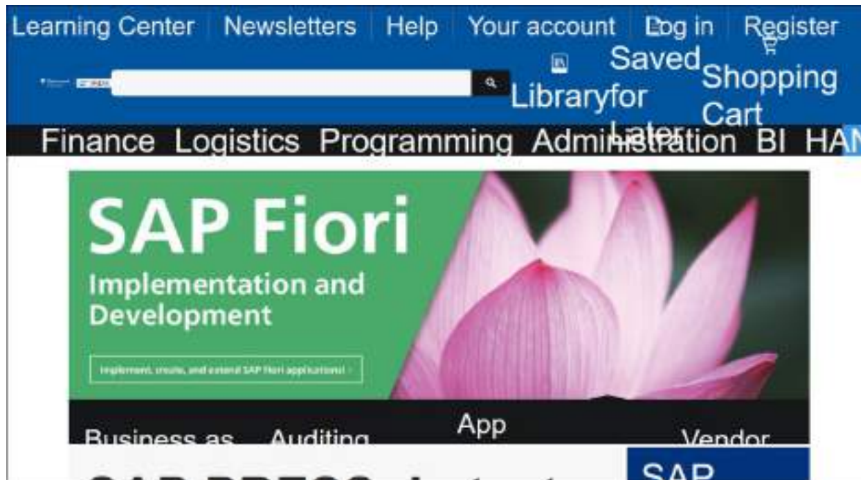
Figure 13.8 Here, the “Zoom Text Only” Function Was Used, but Pixels Were Used for the Layout Wrap in the Media Queries: The Layout Is Gone
