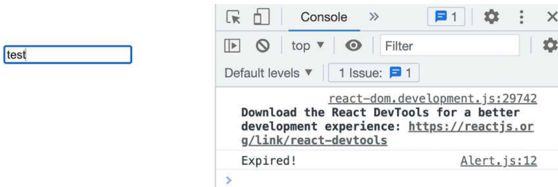
Figure 8.5: The console log does not reflect the entered value
