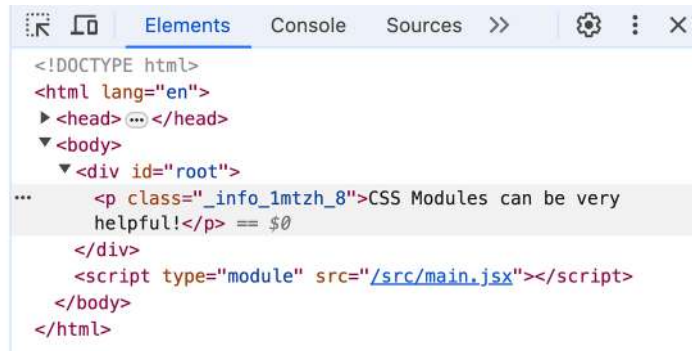
Figure 6.6: CSS class name transforms because of CSS Modules usage
