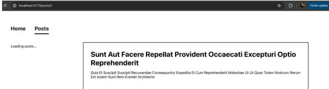
Figure 14.8: Post details are already visible while the list of posts is loading
