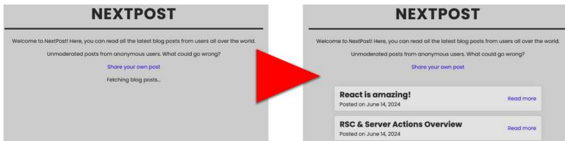
Figure 17.9: Fallback content is shown while the blog posts are fetched
