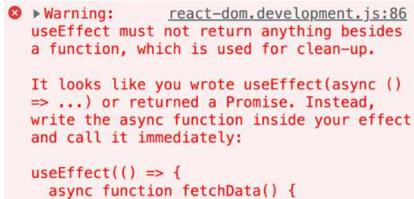
Figure 8.8: React shows a warning about async being used in an effect function
