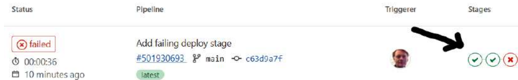
Figure 4.3 – Status icons for a pipeline instance's stages
