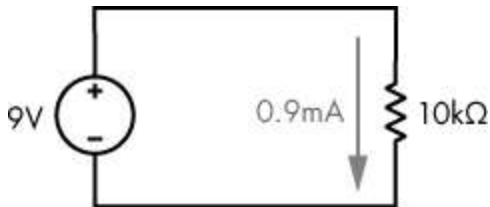
Figure 3-4: A 9-volt battery with a 10,000 \Omega resistor attached across its terminals
