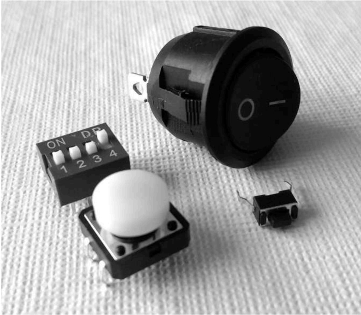
Figure 4-2: Some electrical switches
