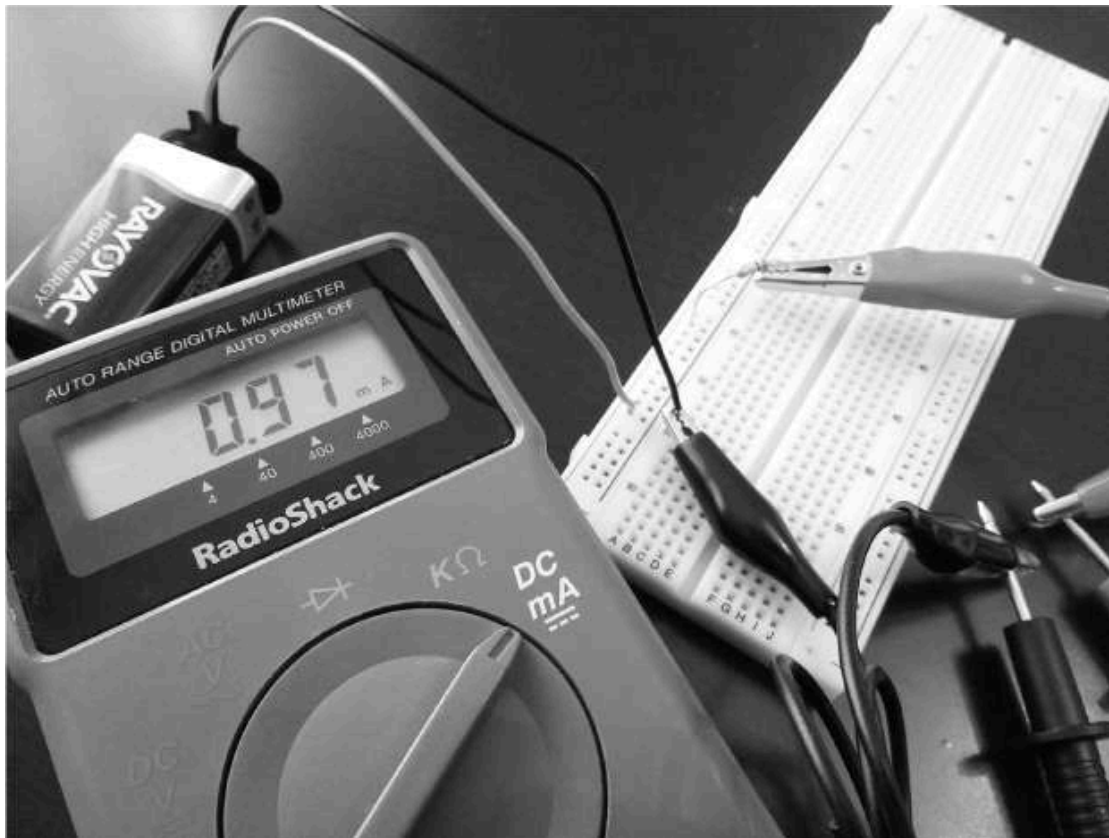
Figure 3-24: Measuring current. The right side of the resistor and the black wire from the battery don't need to be connected to the breadboard.
