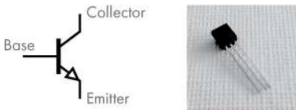
Figure 4-5: The symbol for (left) and photo of (right) an NPN transistor
