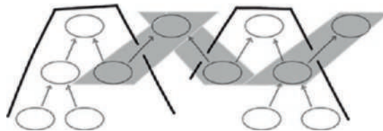
Figure 11-8. The facts downloaded to a device include the cone of successors of a root and all of their predecessors
