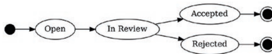
Figure 8-7. The state transition diagram of a commit, as implemented in a separate tool
