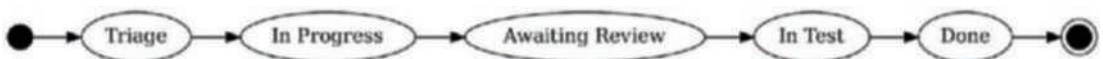
Figure 8-6. The state transition diagram for a software defect, modified to ensure changes are reviewed
